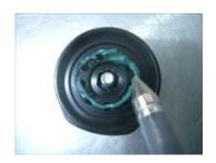
7. Lightly grease detents on underside of U-turn adjuster knob before refitting. Using 2.5mm allen key tighten U-turn knob in position
