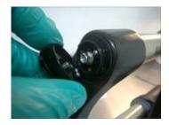
Using a 2.5mm allen key remove U-Turn adjuster knob taking care not to lose the 3 ball bearings & detent springs (tip: use a magnet)
