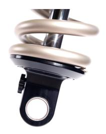
Caution: the adjustment is always made from the closed/screwed down position and the number of clicks is counted.
