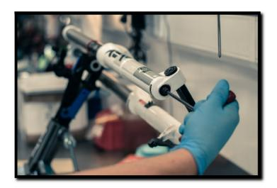
4: Using a soft mallet, tap the foot-nuts to separate the lowers from the stanchions, then undo them fully and set them aside.
