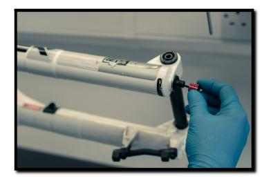
3: Attach the fork horizontally in a steady grip, and undo the foot-nuts, but not all the way out.
