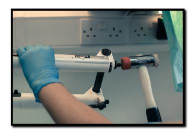
5: You should now be able to pull the lowers from the stanchions, and drain the old lower lube into an appropriate container for safe disposal. Push an old rag through the lowers to make sure they're entirely clean and there's no oil left over.
