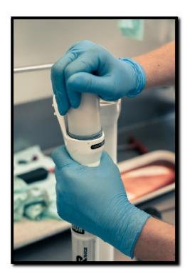
7: Slide the lowers back onto the stanchions, being careful not to fold the lip of the seal as you're sliding them on. Don't slide the lowers all the way up the stanchions yet.
