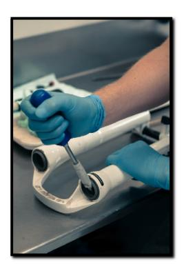
7: When replacing the foams, soak them in lube to ensure smooth operation later on.
