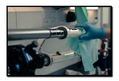
2: Remove the rebound adjuster so you can get at both foot-nuts. On some forks, it is an interference fit and can be pulled out by hand, and on others you have to remove a clip first - check this in your manual before continuing.
