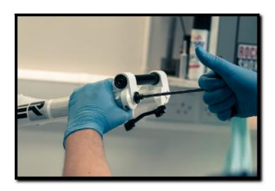
10: Replace the rebound adjuster assembly and refit the fork.
