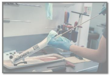
6: If needed you can now replace the seals and foams. Start by carefully levering the wiper seals out of the lowers, then lift the oil seals and foams out.
