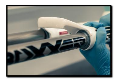
8: Check your manual and measure out an appropriate amount of lube. Squirt the lube into the lowers using the holes at the bottom of each leg. It helps to have the fork at a slight angle for this step, to stop the lube from pouring back out.
