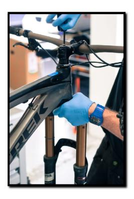
6: Slide any spacers you may have fitted off the stem, and, if you need to, note down which order they were fitted in, i.e. Two above the stem, three below. This will come in handy when you refit your fork.
