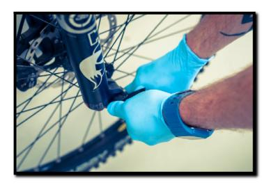
3: Use an allen key to remove the bolts which attach the brake caliper to the fork legs.
