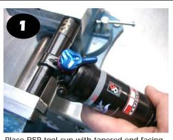
Place RSP tool cup with tapered end facing shock eyelet, slide press shaft through bush and engage in cup.
