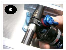
Turn RSP tool cup over so that straight sides are facing shock eyelet, place new bush on press shaft. Line up bush with eyelet and engage drift shaft in cup.
