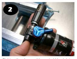
Tighten the vice, pushing out old bush into the RSP tool cup or use a soft-faced hammer to tap the bush out. Remove bush from tool cup.
