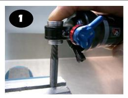
Use an easy-out mounted in a vice to remove the old reducers. Gently press down on the shock while turning anti-clockwise to engage the easy-out helix.
