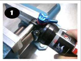
Push steel pin/axle into shock eyelet. To avoid damage to the bush (especially if using DP or DU coated bush) ensure you push it squarely with a vice or tap in gently with a soft-faced hammer.
