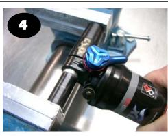
Fit new bush by tightening vice or use a soft faced hammer, ensuring it goes in straight (this is important when fitting a polymer bush otherwise you may shave material off the outside) until it's flush with eyelet.
