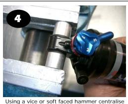
Using a vice or soft faced hammer centralise the shock on the mount kit pin. Re-fit shock into frame and go ride!
