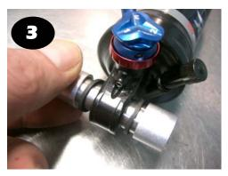
If you have rubber quad rings place one either side of the eyelet. Slide an alloy spacing sleeve onto each side of the steel pin/axle.
