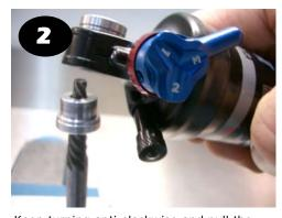
Keep turning anti-clockwise and pull the shock upwards, the reducer should then come out without damaging the shock eyelet. Repeat for other side.
