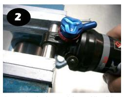
Rotate the shock up and down whilst sliding it across until it's central in the eyelet.
